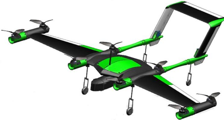
Figure 8 – VTOL configuration of this RPV model.
