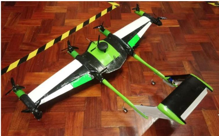
Figure 10 – VTOL final configuration.
