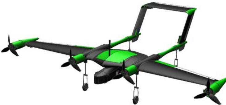
Figure 5 – STOL configuration of this RPV model.
