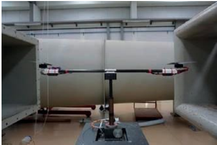
Figure 10: Boom with VTOL system to be tested in the wind tunnel
